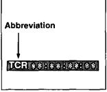
CTL (control signal) (TC time code playback value) TCR UBR (TC user's bit playback value)
