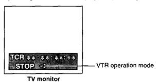
The VTR's major settings are performed by making selections using a menu system. The set-up menus appear on the TV monitor when it is connected to the MONITOR OUT connector.
